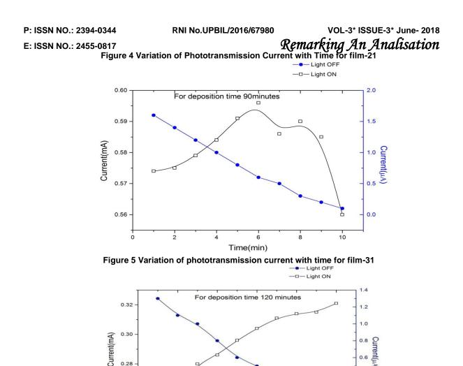
The variation of phototransmission current at the specified distance (30cm) is found to increase with time and then saturates to a almost constant value. When light is switched off, the current starts to fall rapidly and reached a certain minimum value which is approximately same for all the films deposited at different times.
